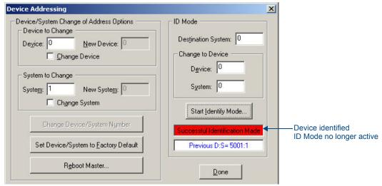
FIG. 20 Device Addressing dialog - Successful Identification Made
